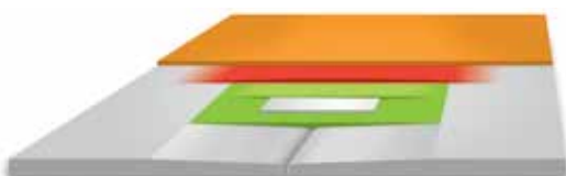
Q2 + 1 layer of plaster over the entire surface of the board
