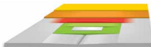
Q3 + 1 layer of ultra-fine plaster over the entire surface of the board
