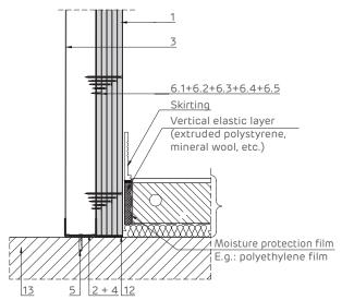
Detailed attachment at the top on reinforced concrete members. Installation height:  $H \le 5$  m.
