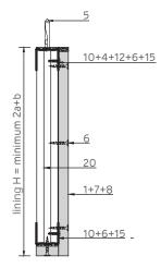
Detail of single side lining. Vertical section
