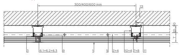
Crossing with D wall less resistant to fire Horizontal section.
