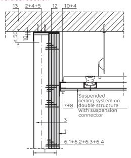
Lining of a wooden item Horizontal section.
