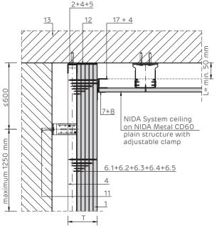
NIDA Metal UD runner profile may not be fixed to the wall structure in the plasterboard sliding area.
