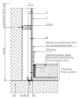
Detailed crossing with suspended ceiling on plain structure with adjustable clamp. Vertical section
