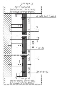
Detailed crossing with suspended ceiling on plain structure with adjustable clamp. Vertical section
