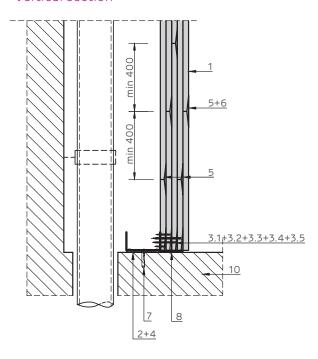
NIDA plasterboards are to be mounted long-sided horizontally, using one-piece boards!!! Vertical joints between plasterboards are not allowed in the field area of the lining!!!
