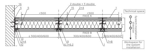
Lining crossing with D wall less resistant to fire. Horizontal section.
