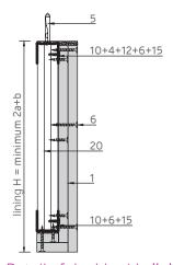
Detail of double side lining. Vertical section
