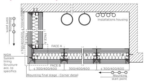
Two-sided enclosing of installations housing Horizontal section.
