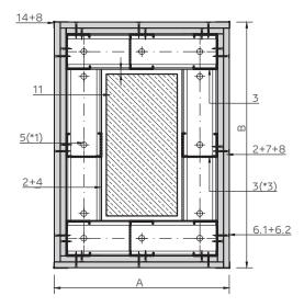
(\*1) A minimum of 3 fasteners should be fitted along NIDA Metal UD. (\*3) If the lining size (A/B) exceeds the maximum value of 600 mm, an additional upright (marked with a dotted line in the plan) should be placed.
