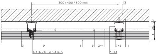
Crossing with D wall less resistant to fire Horizontal section.
