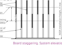
Board staggering. System elevation. Vertical and horizontal joints should be staggered to avoid overlap.
