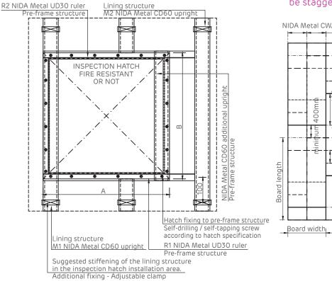
Board staggering. System elevation. Vertical and horizontal joints should be staggered to avoid overlap.
