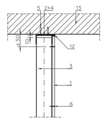
Lining of a wooden item Horizontal section.
