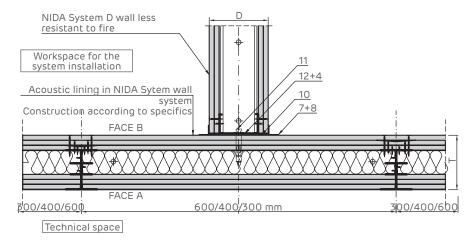
Lining crossing with D wall more resistant to fire. Horizontal section.
