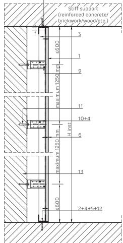
A minimum of 3 fasteners should be fitted along NIDA Metal UD. (\*3) If the lining size (A/B) exceeds the maximum value of 600 mm , an additional upright ( marked with a dotted line in the plan) should be placed.
