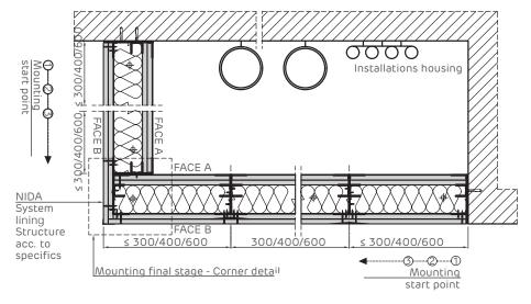
Two-sided enclosing of installations housing Horizontal section.
