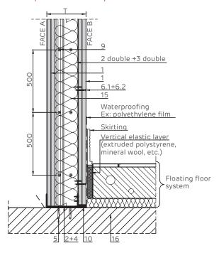
Upper fastening detail on reinforced concrete slab.
