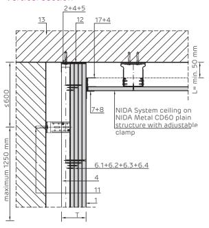
NIDA Metal UD runner profile may not be fixed to the wall structure in the plasterboard sliding area.
