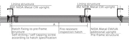
The detail presented is general in nature and focuses on the stiffening of the structure in the hatch installation area. It will be customised according to the model of hatch to be installed in the NIDA system
