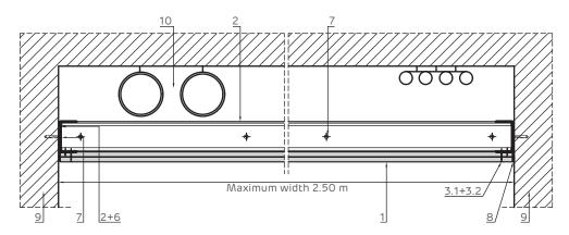
NIDA plasterboard mounting details. Joint staggering - Vertical section.
