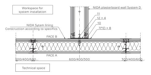
Lining crossing with D wall more resistant to fire. Horizontal section.
