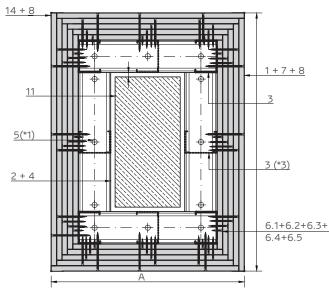
(\*1) A minimum of 3 fasteners should be fitted along NIDA Metal UW profile (\*3) If the lining size (A/B) exceeds the maximum value of 600 mm, an additional upright (marked with a dotted line in the plan) should be placed
