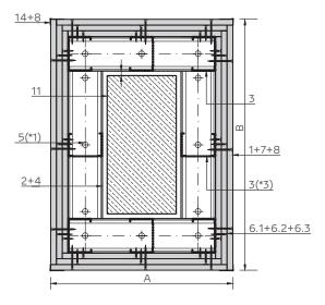
(\*1) A minimum of 3 fasteners should be fitted along NIDA Metal UD. (\*3) If the lining size (A/B) exceeds the maximum value of 600 mm, an additional upright (marked with a dotted line in the plan) should be placed.
