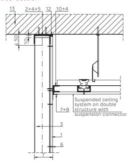
Detailed attachment at the top on reinforced concrete members. Installation height:  $H \le 5$  m. Vertical section.
