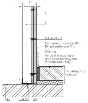
Detailed attachment at the top on reinforced concrete members. Installation height:  $H \le 5$  m. Vertical section.
