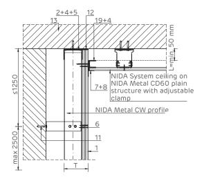
NIDA Metal UD runner profile may not be fixed to the wall structure in the plasterboard sliding area.
