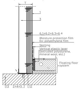
Detailed attachment at the top on reinforced concrete members. Installation height: H ≤ 5 m. Vertical section.
