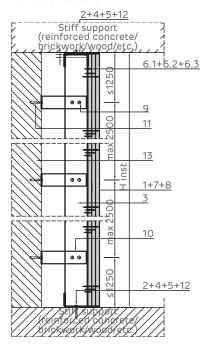
Detailed crossing with suspended ceiling on plain structure with adjustable clamp. Vertical section
