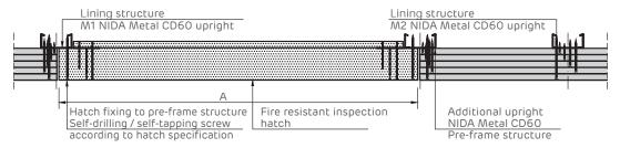
The detail presented is general in nature and focuses on the stiffening of the structure in the hatch installation area. It will be customised according to the model of hatch to be installed in the NIDA system
