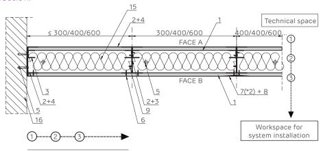
NIDA System T - Acoustic lining in wall system lining with single board layer on NIDA Metal UW/UD structure Horizontal section.
