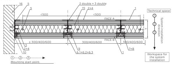
Lining crossing with D wall less resistant to fire. Horizontal section.
