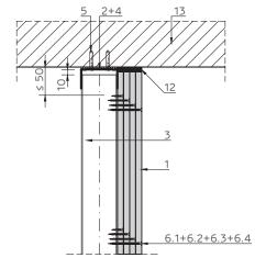
Detailed crossing with suspended ceiling on double structure with adjustable clamp. Vertical section
