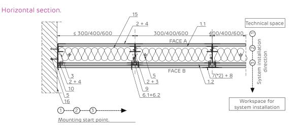
Lining crossing with D wall less resistant to fire or not resistant at all Horizontal section.
