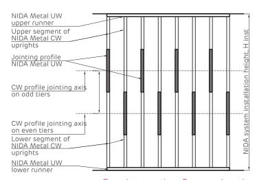
Board staggering. System elevation. Vertical and horizontal joints should be staggered to avoid overlap
