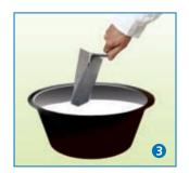
Mixing must be done in a perfectly clean plastic or rubber pot and the water must be clean and come from, for example, the drinking water supply. The temperature of the water and the environment must be above  $5^{\circ}$ C. NIDA Boardfix adhesive plaster should be prepared according to the instructions on the back of the bag and in the data sheet.
