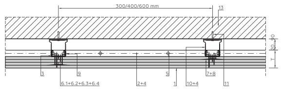
Crossing with D wall less resistant to fire Horizontal section.
