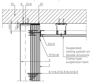
Lining of a wooden item Horizontal section.
