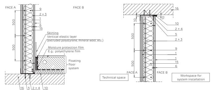
Three-sided enclosing of installations housing. Horizontal section.
