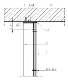
Detailed crossing with suspended ceiling on double structure with suspension connector. Vertical section
