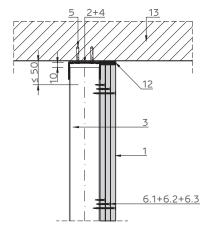
Detailed crossing with suspended ceiling on double structure with adjustable clamp. Vertical section
