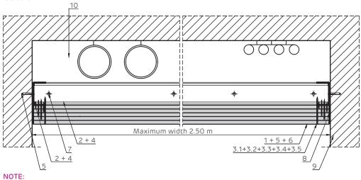
NIDA plasterboards are to be mounted long-sided horizontally, using one-piece boards!!! Vertical joints between plasterboards are not allowed in the field area of the lining!!!
