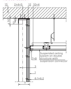
Lining of a wooden item Horizontal section.
