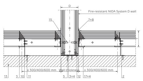
Detailed attachment at the top on the roof profiled sheet. System perpendicular to the profiles. Vertical section
