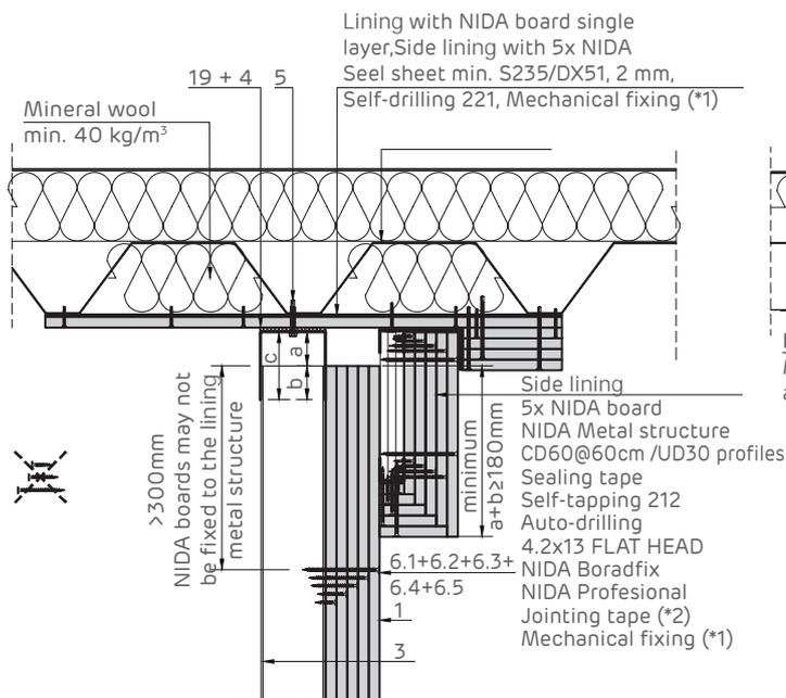
Detailed attachment at the top to the roof profiled
