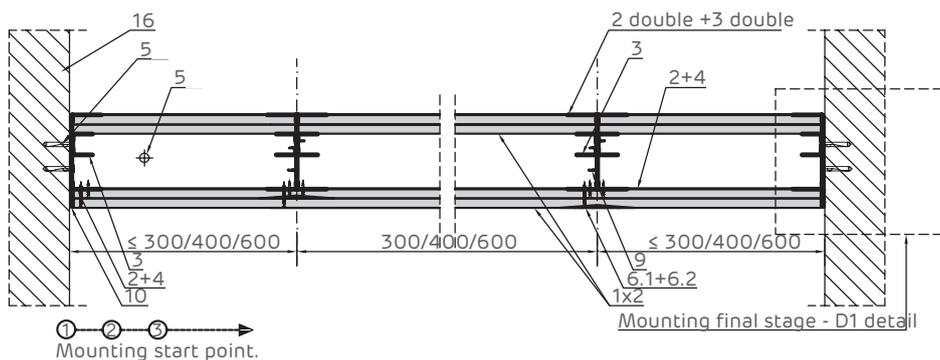
The system should be mounted from one end in the case of linear lining, fixed between two enclosing elements (e.g. brick wall, reinforced concrete). In the case of lining of technical spaces which are L-shaped or U-shaped, the system should be mounted in such a way that it closes at all times in the corner area
