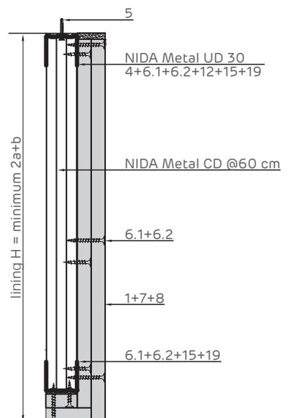
Sliding attachment detail at top on reinforced concrete members. Vertical section
