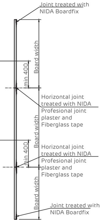
NIDA plasterboard mounting details. Joint stagger.
