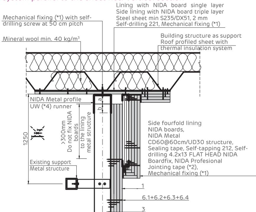
Detail of double side lining. Vertical section
