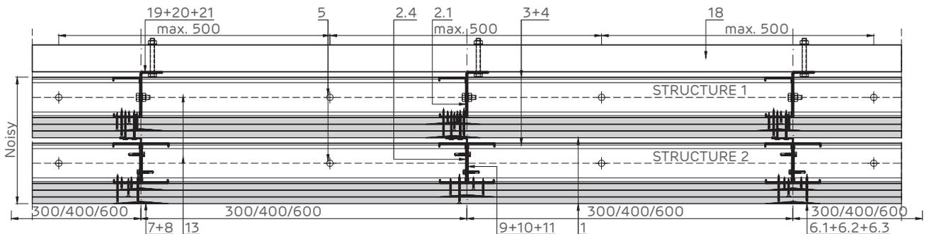
Horizontal section: Double upright for Structure 1 and Structure 2
