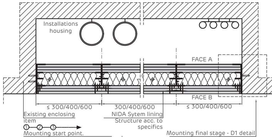
Two-sided enclosing of installations housing Horizontal section.
