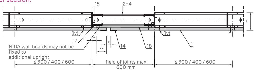
(\*) The size of the joint will also be determined by the size of the structural joint, but not less than 20 mm
