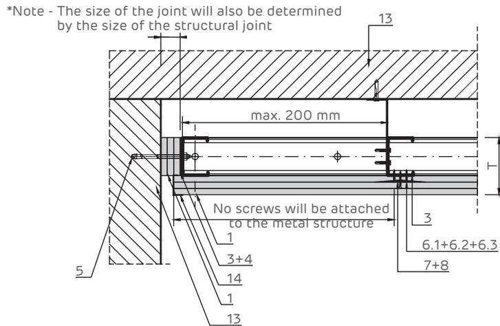
Detailed attachment at the top on the roof profiled sheet System parallel to the sheet ribs. Vertical section
