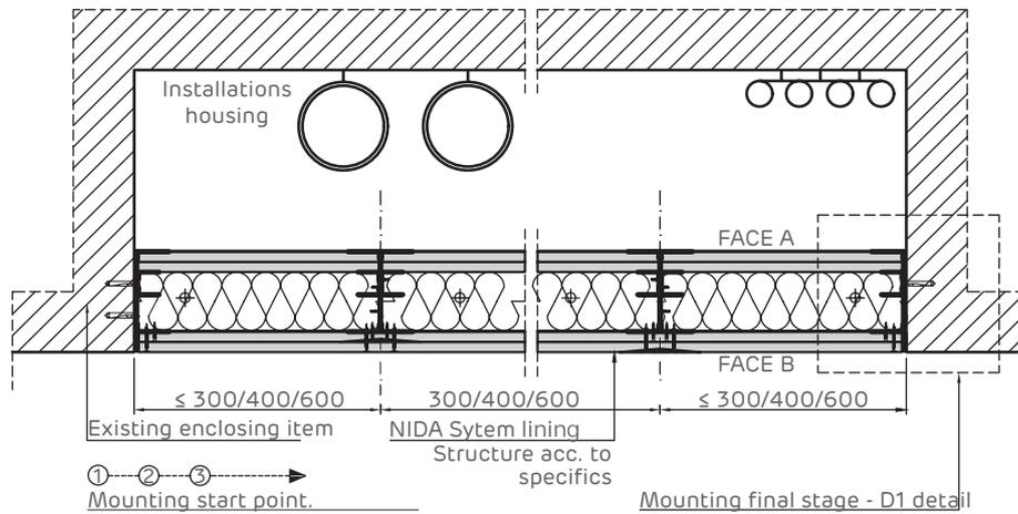
Two-sided enclosing of installations housing Horizontal section.
