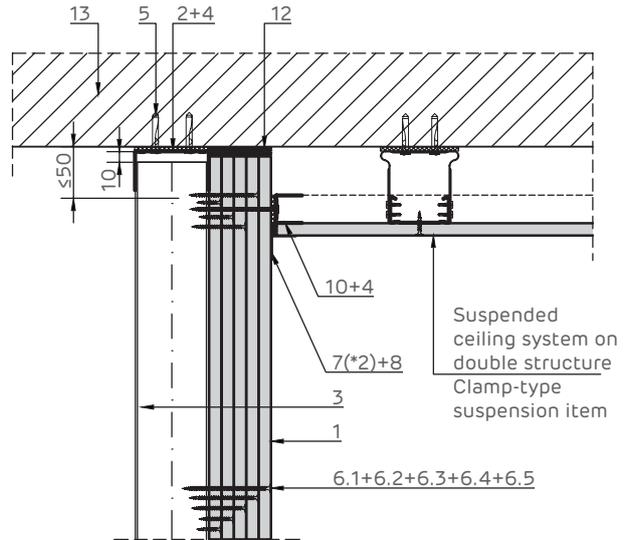
Lining of a wooden item Horizontal section.
