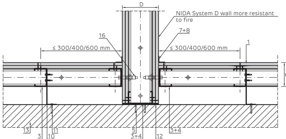
Detailed attachment at the top on the roof profiled sheet.
