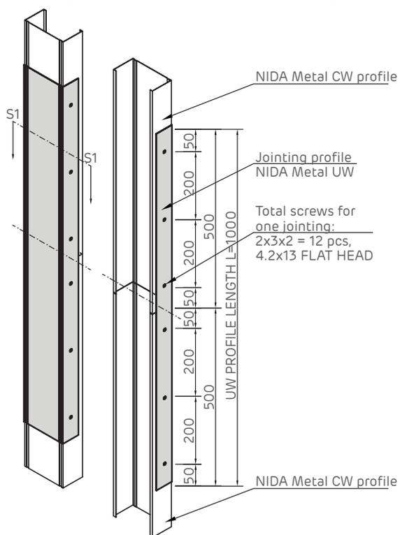
Jointing detail of NIDA Metal CW double profiles.
