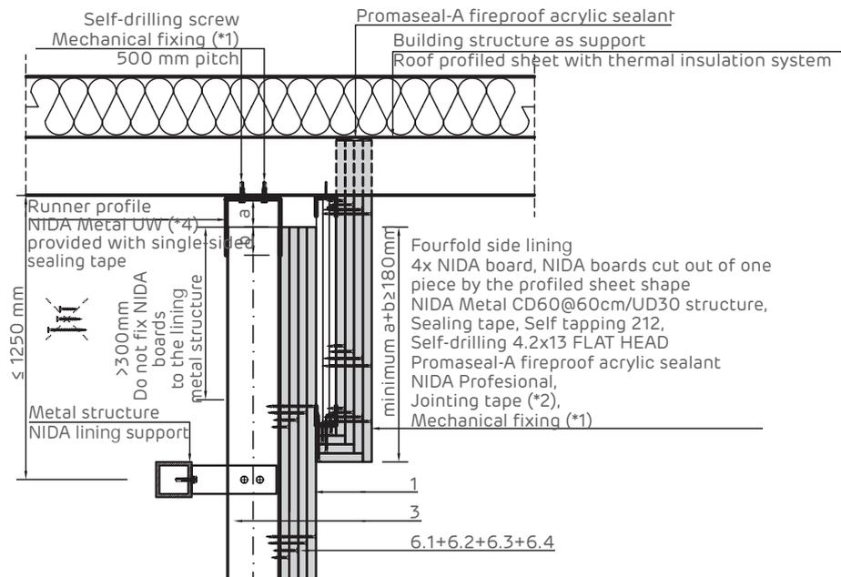
Access hatch elevation.
