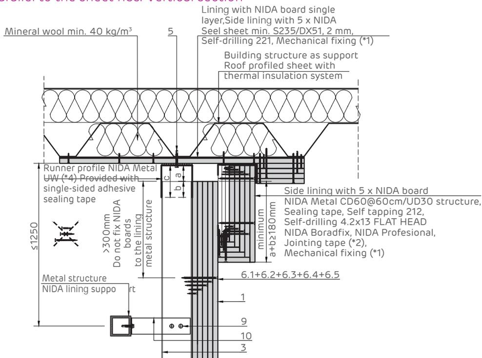
Sliding attachment detail at top on reinforced concrete members. Vertical section
