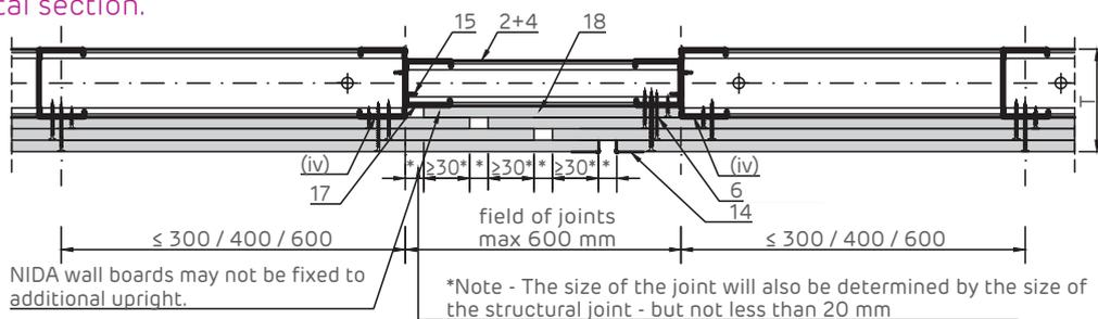
(\*) The size of the joint will also be determined by the size of the structural joint, but not less than 20 mm
