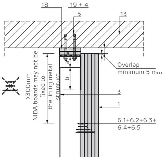
Detailed crossing with suspended ceiling on double structure with adjustable clamp. Vertical section
