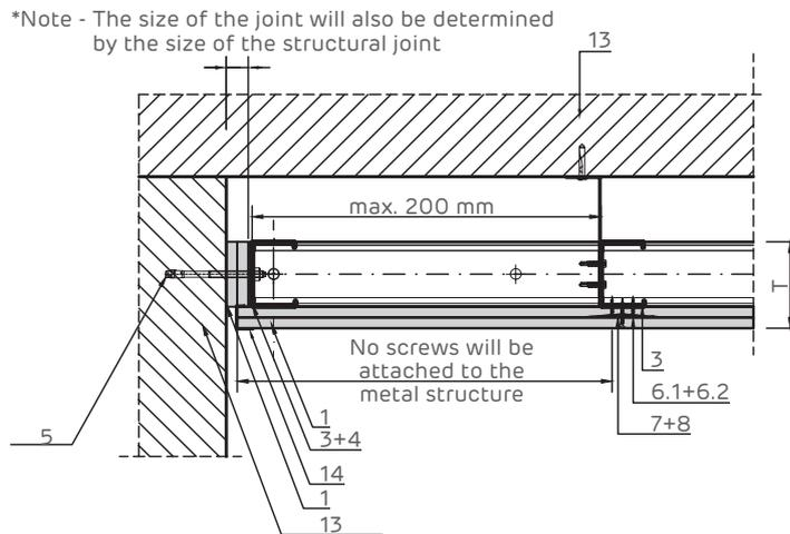
Detailed attachment at the top on the roof profiled sheet. System parallel to the sheet ribs. Vertical section
