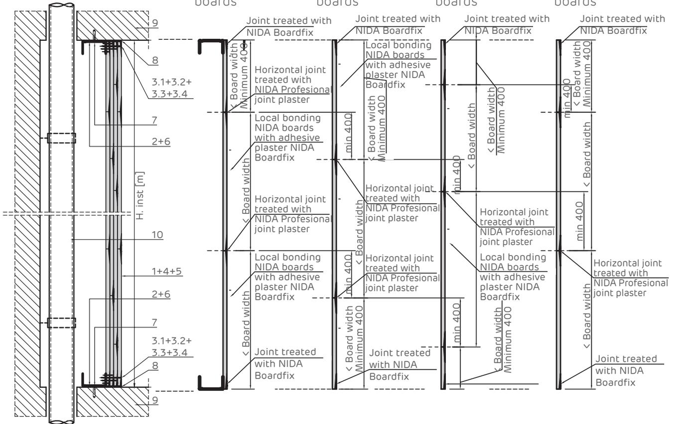
NIDA plasterboard mounting details. Joint stagger.
