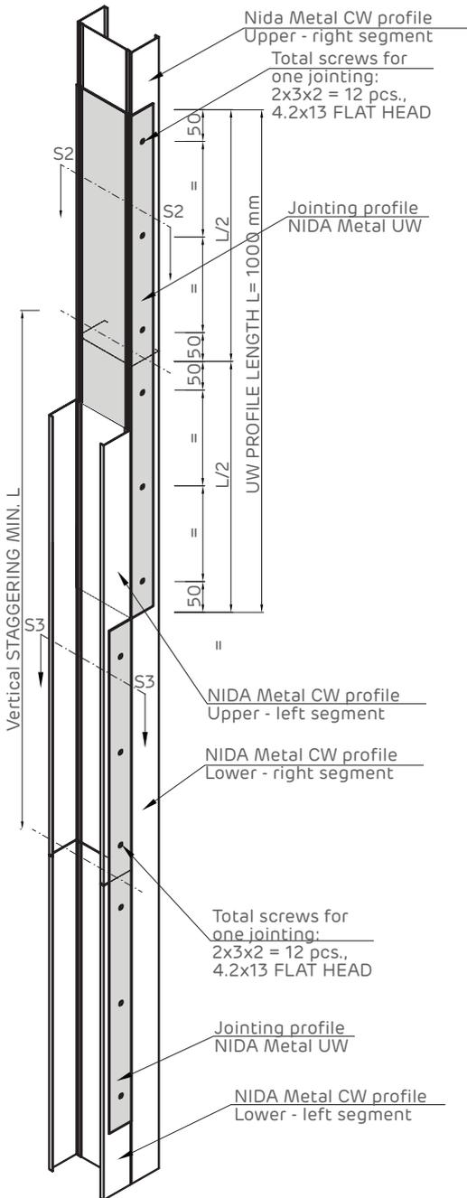
NIDA Metal CW profile joint staggering System elevation.
