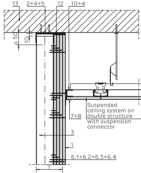
Detailed attachment at the top on reinforced concrete members.
