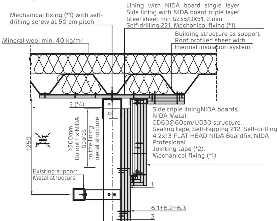
Detail of double side lining. Vertical section
