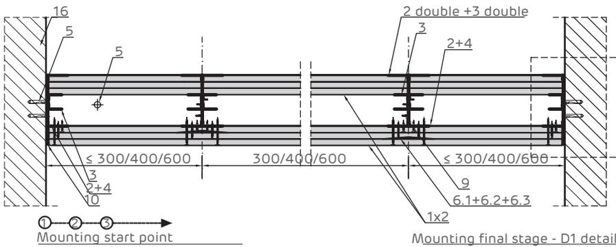
The system should be mounted from one end in the case of linear lining, fixed between two enclosing elements (e.g. brick wall, reinforced concrete). In the case of lining of technical spaces which are L-shaped or U-shaped, the system should be mounted in such a way that it closes at all times in the corner area
