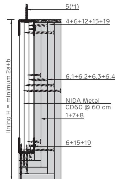
Sliding attachment detail at top on reinforced concrete members. Vertical section
