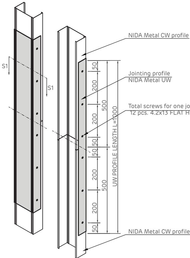
Joining detail of NIDA Metal CW double profiles.
