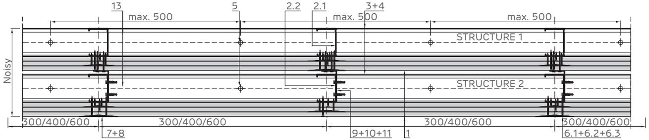
Horizontal section: Double upright for Structure 1 and single upright for Structure 2
