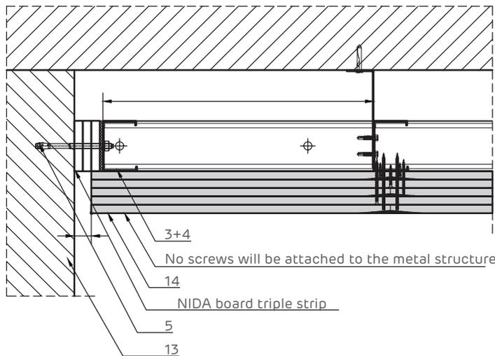
Detailed attachment at the top on the roof profiled sheet. System parallel to the sheet ribs. Vertical section
