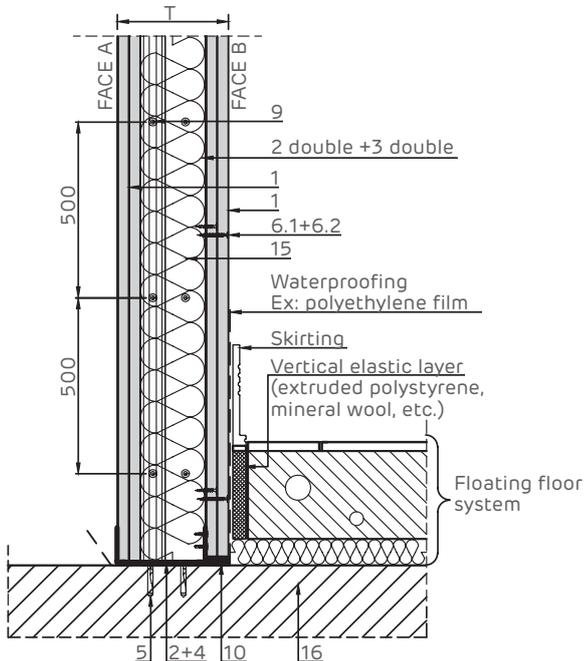
Upper fastening detail on reinforced concrete slab.
