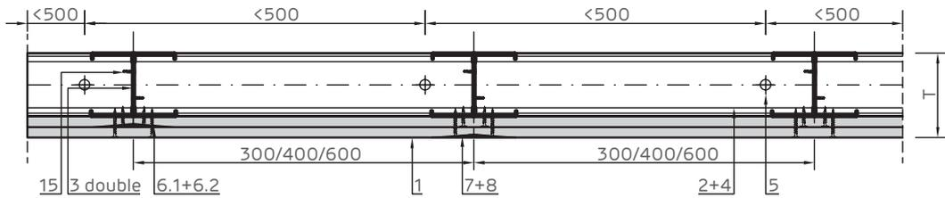
Three-sided enclosing of installations housing Horizontal section.
