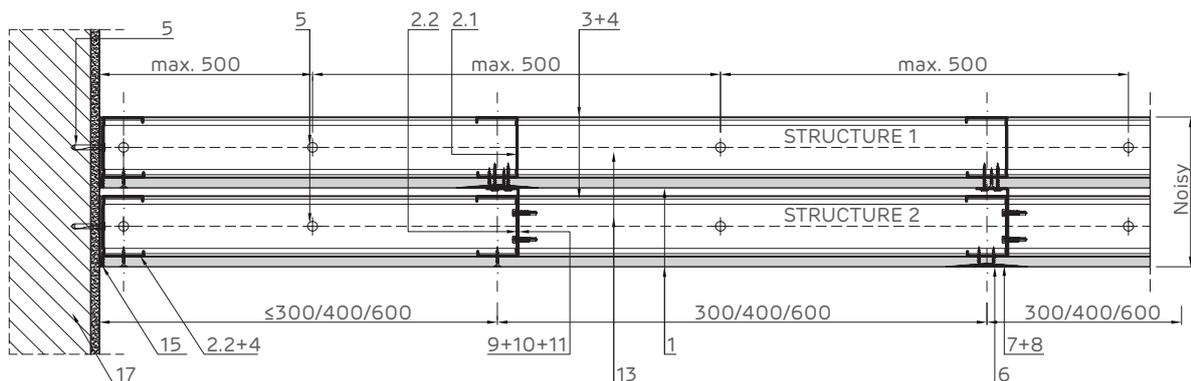
Jointing detail of NIDA Metal CW double profiles.
