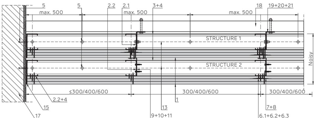
Jointing detail of NIDA Metal CW double profiles.
