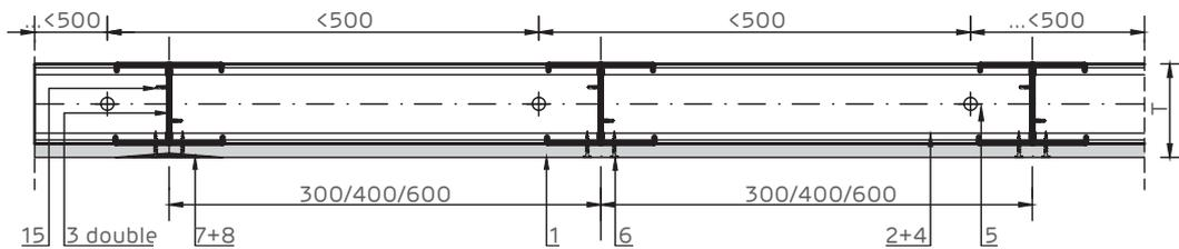
Three-sided enclosing of installations housing Horizontal section.
