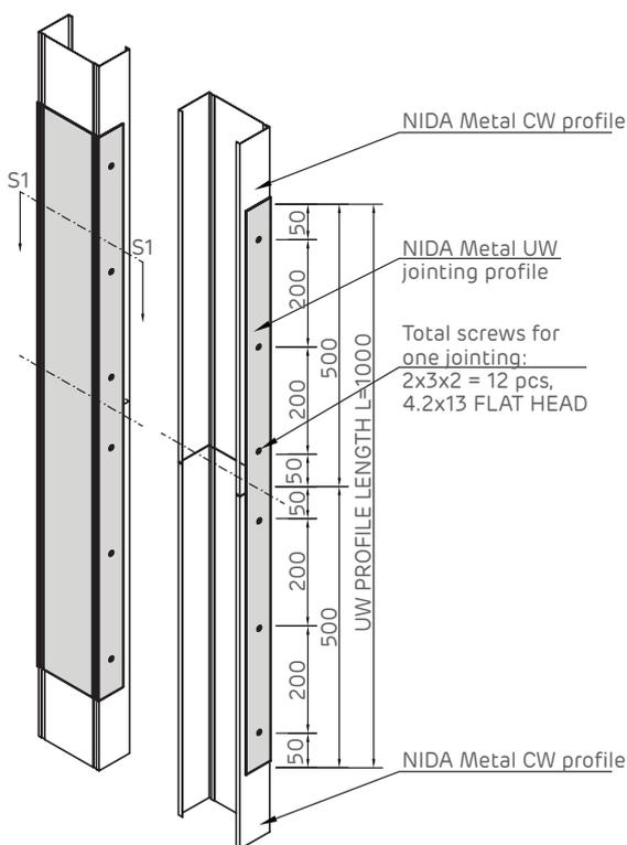
Joining detail of NIDA Metal CW doubled profiles.
