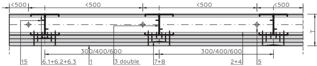
Three-sided enclosing of installations housing Horizontal section.
