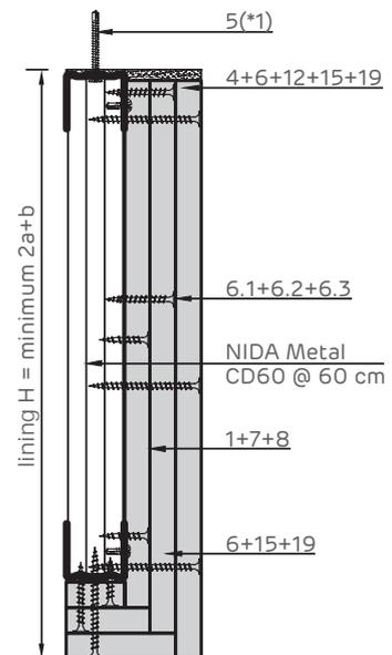
Sliding attachment detail at top on reinforced concrete members. Vertical section
