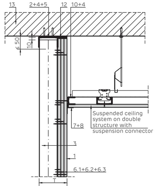
Detailed attachment at the top on reinforced concrete members.
