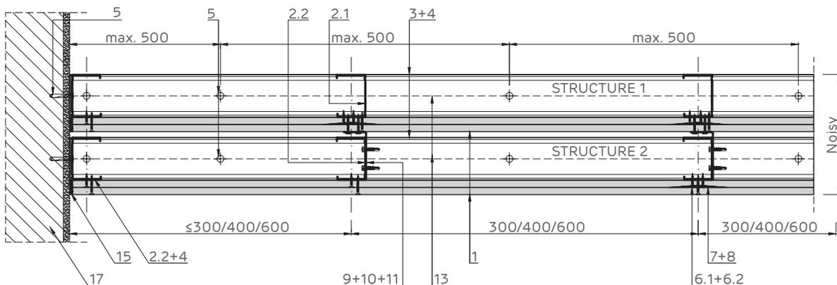
Jointing detail of NIDA Metal CW double profiles.
