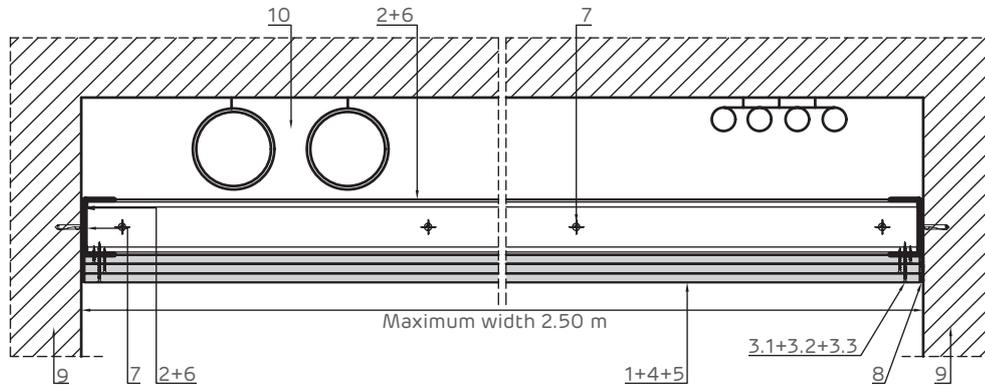
NIDA plasterboard mounting details. Joint staggering - Vertical section.
