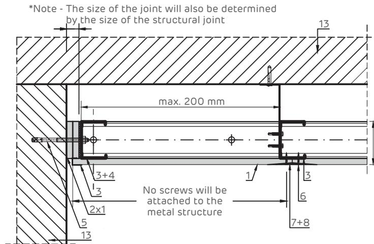
Detailed attachment at the top on the roof sheet. System parallel to the sheet ribs. Vertical section
