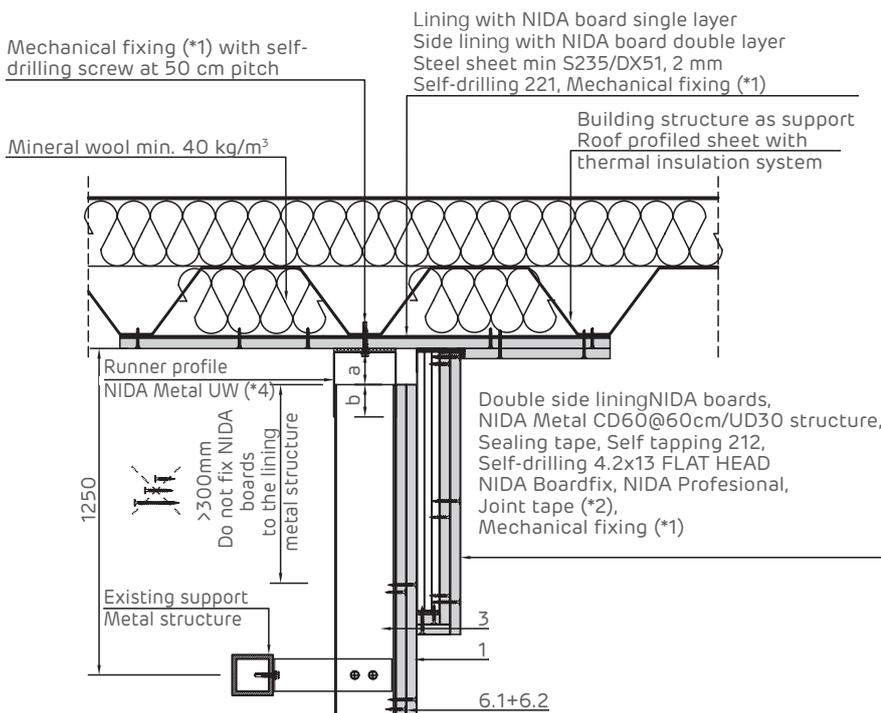
Detail of double side lining. Vertical section
