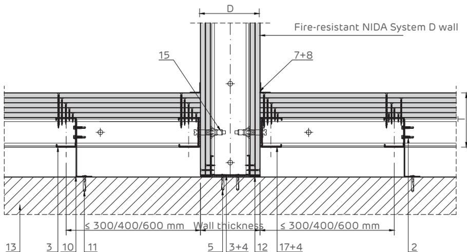
Detailed attachment at the top on the roof profiled sheet.
