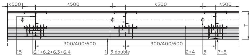
Three-sided enclosing of installations housing Horizontal section.
