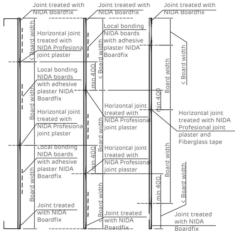
NIDA plasterboard mounting details. Joint stagger.
