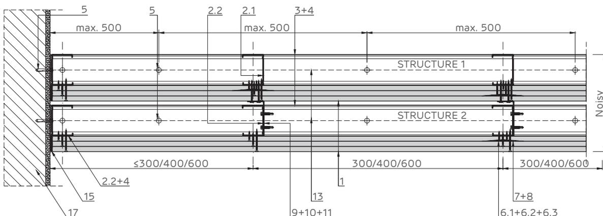
Jointing detail of NIDA Metal CW double profiles.
