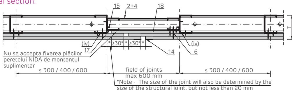
(\*) The size of the joint will also be determined by the size of the structural joint, but not less than 20 mm
